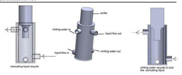
316 stainless steel with double walls through which cooling water can circulate,
